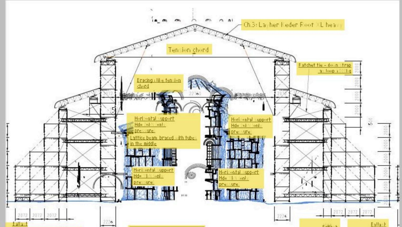
All joints of standards have to be secordes with bolts or hinged pins!
