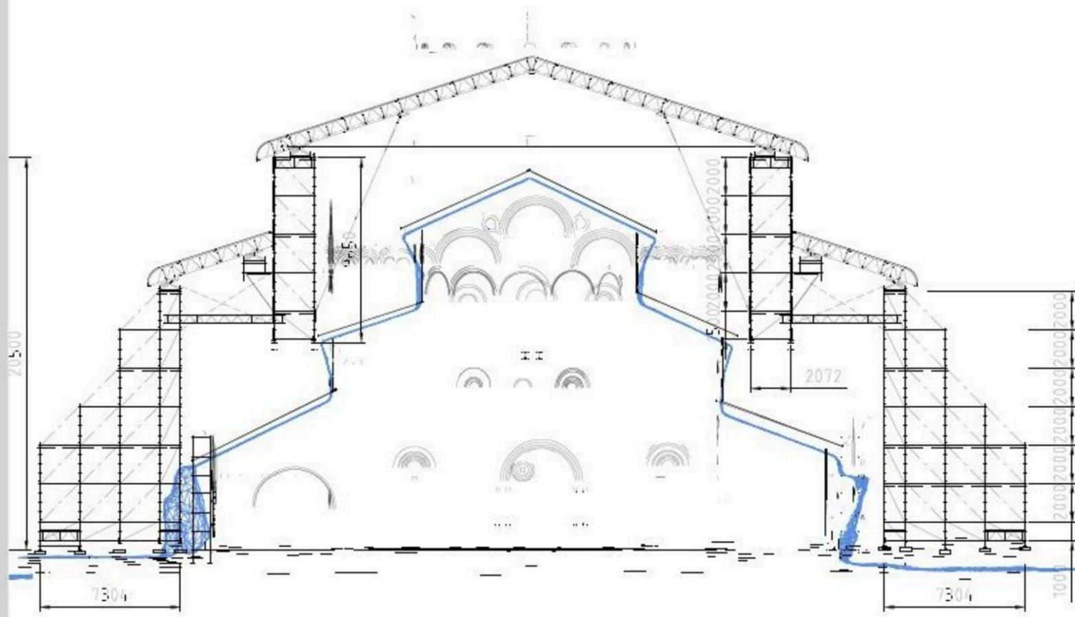
Steel beams, ratchet tie-down strap and ballast are to be provided on site, according to Knobloch Consulting Engineers.
