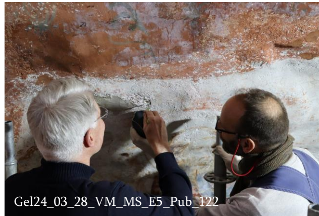
Left: The process of sampling the stratigraphy through core sampling to determine the composition of salts.
