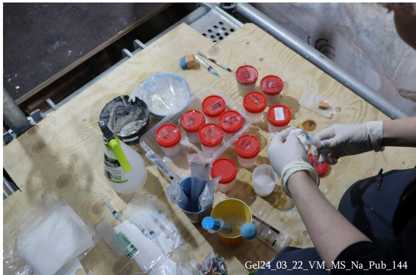
Above: Application of consolidant via syringe and need to allow conservation material penetrate in powdered substrate in pointed areas; Images present process of testing different consolidating materials.
