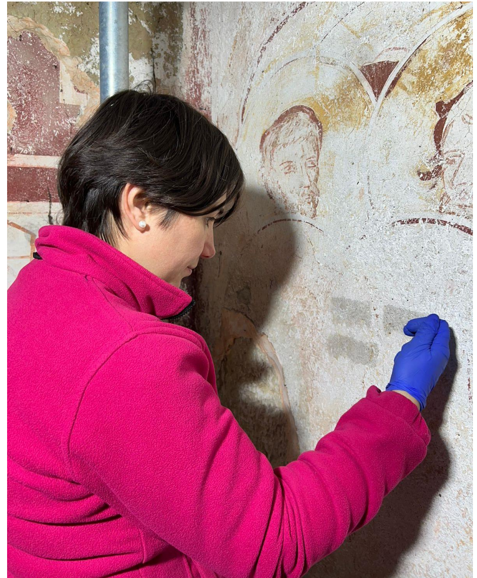
Above: Application of consolidant via syringe and need to allow conservation material penetrate in powdered substrate in pointed areas; Images present process of testing different consolidating materials.
