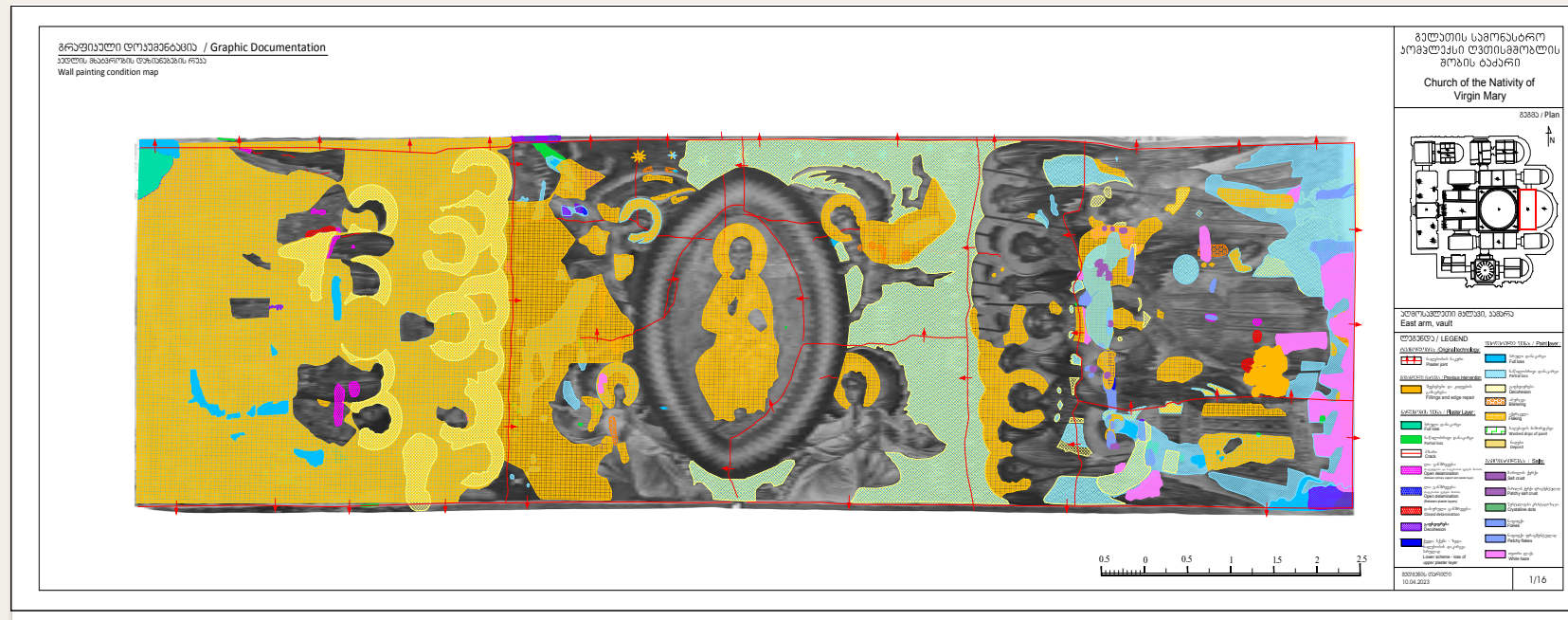
Above: An example of the graphic documentation of conditions being carried out for all the Gelati wall paintings, providing a comprehensive record of their state of conservation.
