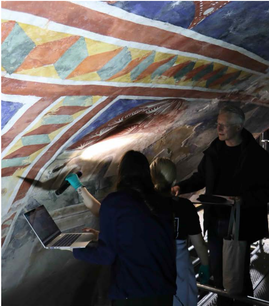
Above: Professor Dr Steffen Laue (Fachhochschule Potsdam, University of Applied Sciences) with members of the conservation team monitoring and sampling salts in the West Arm.
