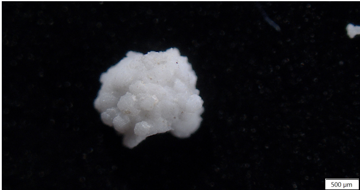
Fig. I-27: Sample 24: white granular crystals agglomerated to a crust, here cauliflower like
