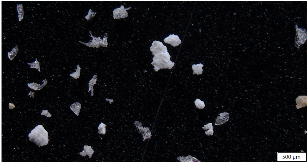
Fig. I-23: Sample 22: white flakes and transparent whisker
