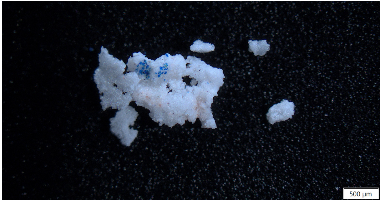
Fig. I-5: Sample 13: white crust with blue particles
