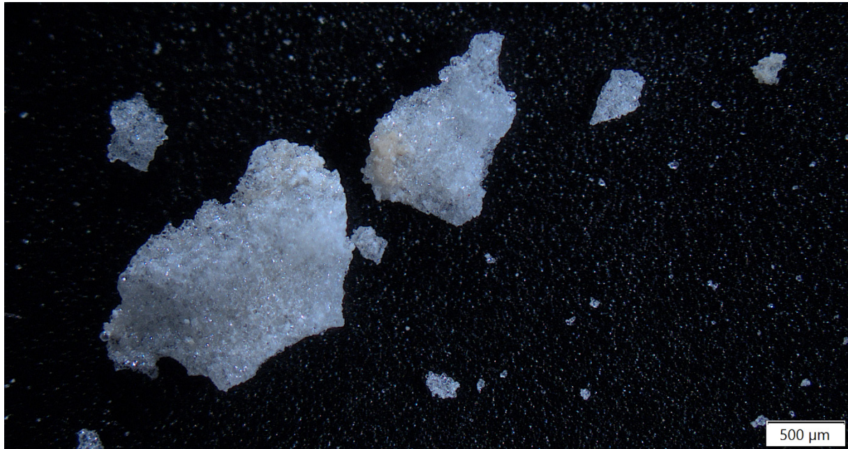
Fig. I-9: Sample 15: granular crystals agglomerated to a white crust
