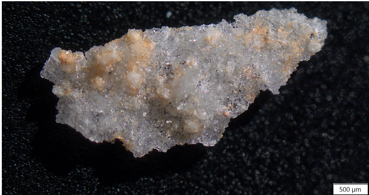
Fig. I-11: Sample 16: granular crystals agglomerated to a crust with ochre particles
