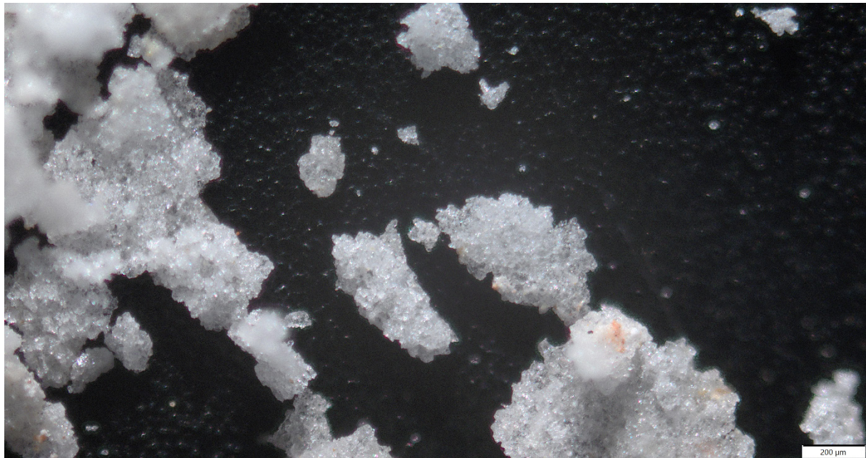
Fig. I-25: Sample 23: granular crystals agglomerated to a crust
