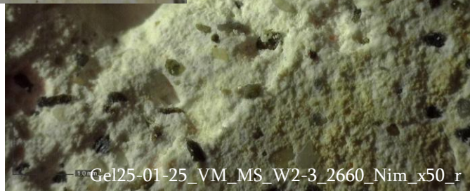
Above: Microscopic composition of the aggregate (at 50x magnification). The white binder uses inorganic sand aggregates of various colors and morphologies.
