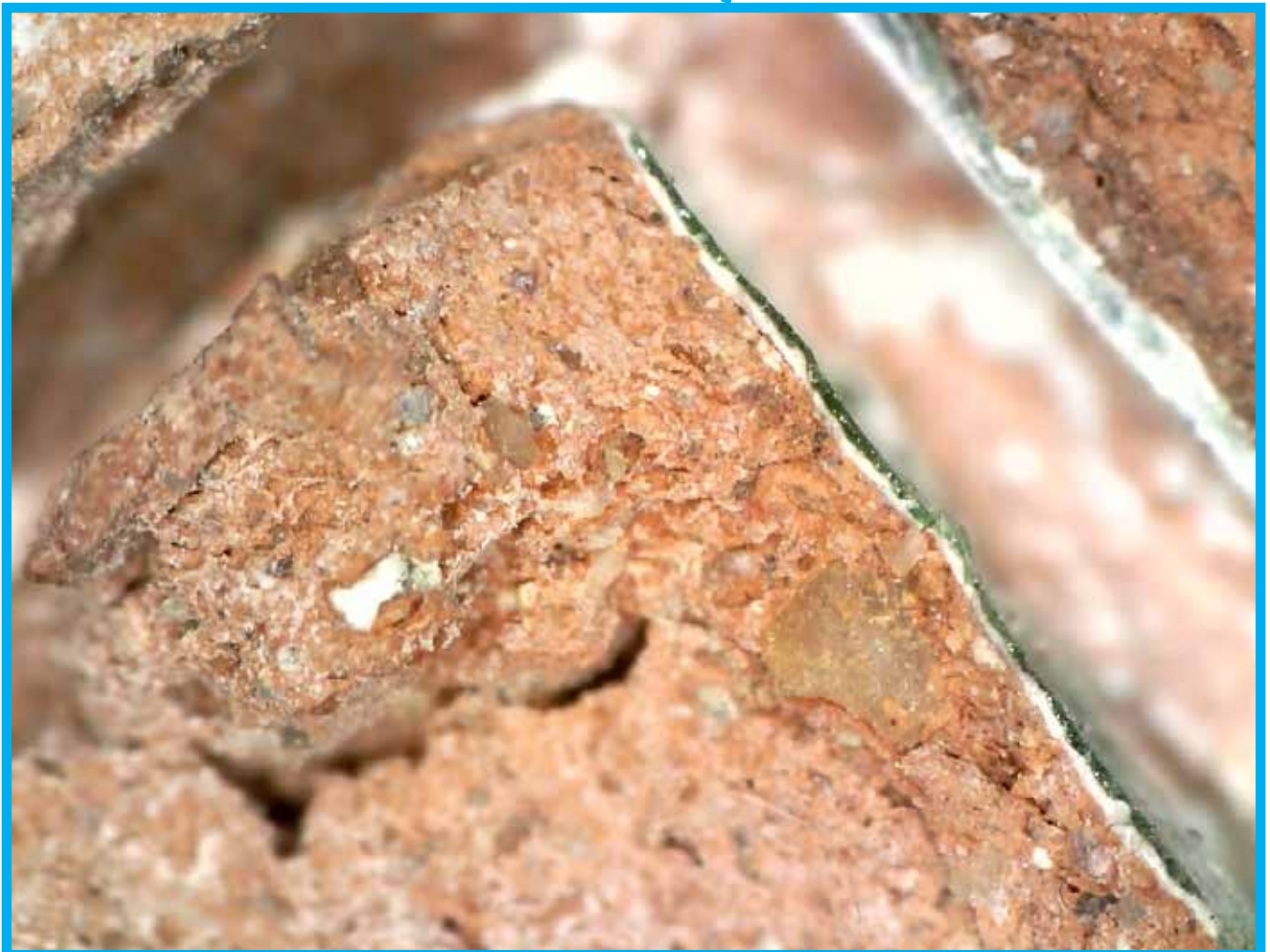
36. A detail with dinolite photograph of a terracotta tessera
