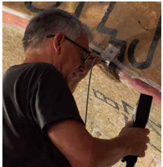
29-30. In order to investigate the hollow spaces behind the mosaic, a video borescope was used.
