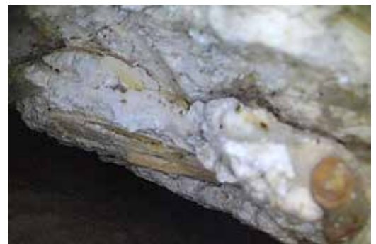
8-9. Details of straw elements embedded into the mortar
