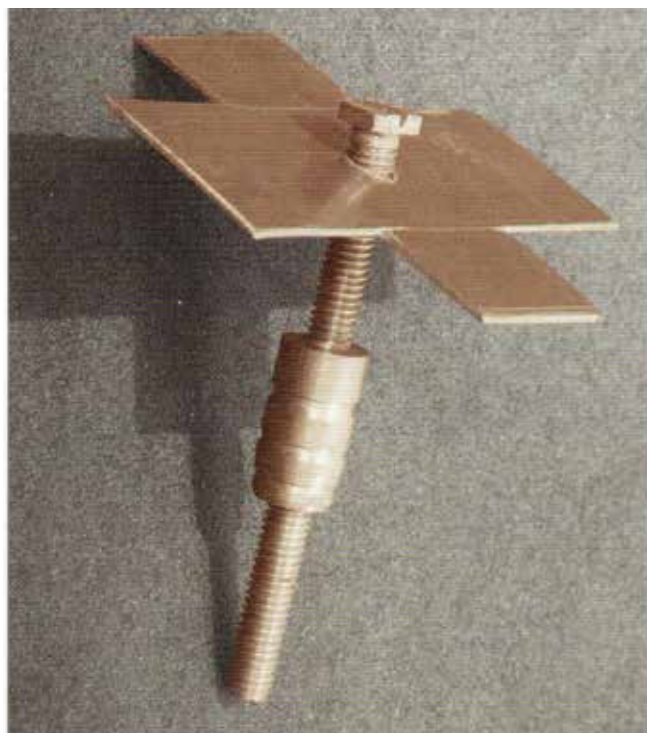
20. An example of the brass pins used during the restoration of the '80s
