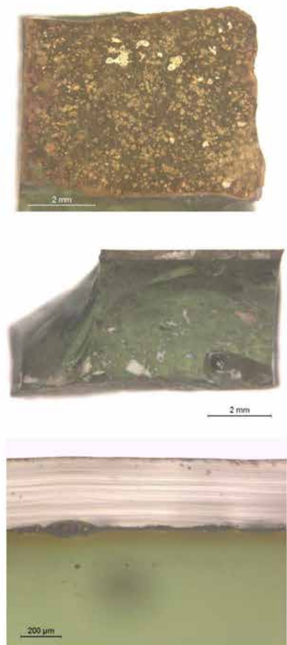
Optical microscope photo of AREA 14 sample 14; from top to bottom: front, side and polished side at different magnifications
