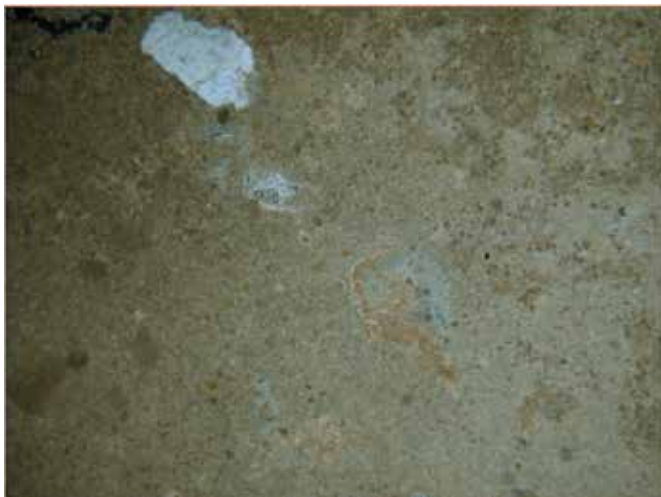
7. Lime lumps and very rare aggregates with porosity in photo. MPOM photomicrograph in transmitted light, thin section, 80 x N+.
