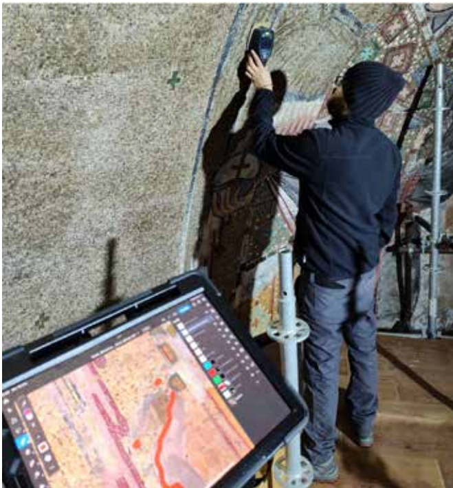
34-35. The geo-radar investigation carried out in a "targeted" way, instead of an extensive way.
