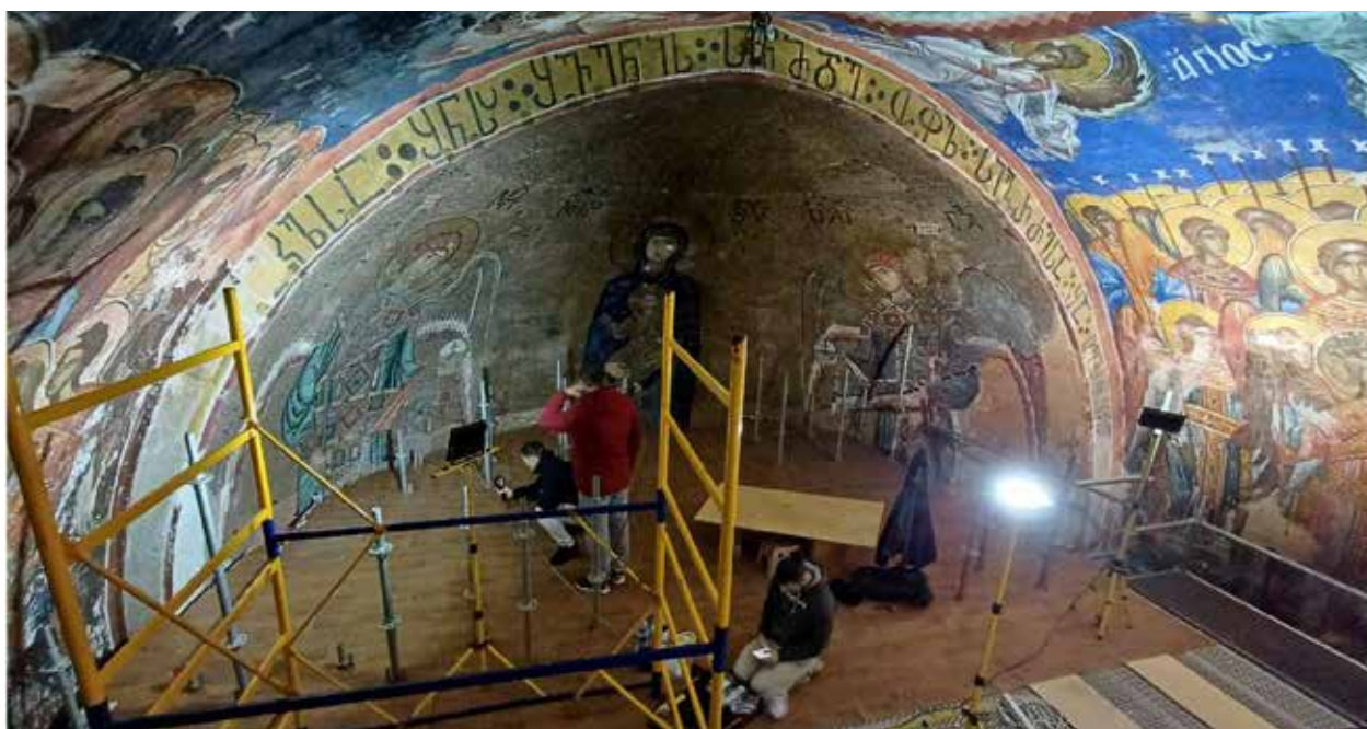
33. The geo-radar survey carried out to identify internal metal elements
