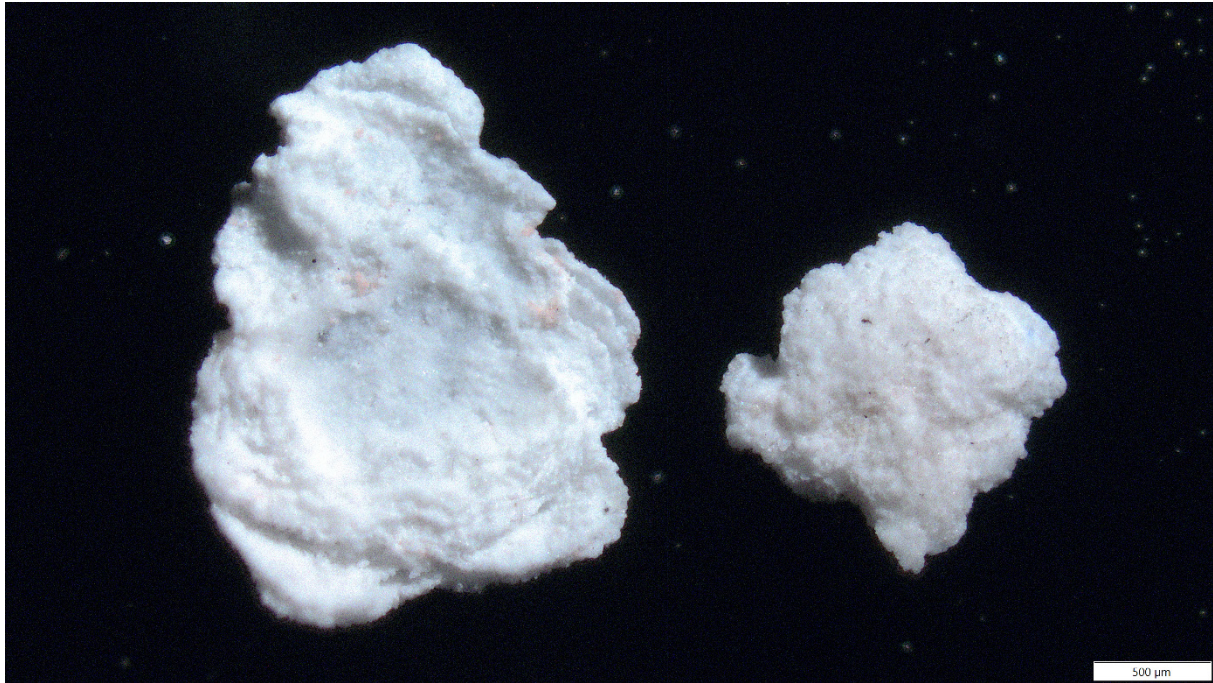
fig. 5: Sample 3.1, thin white crusts with some reddish particles (DF)
