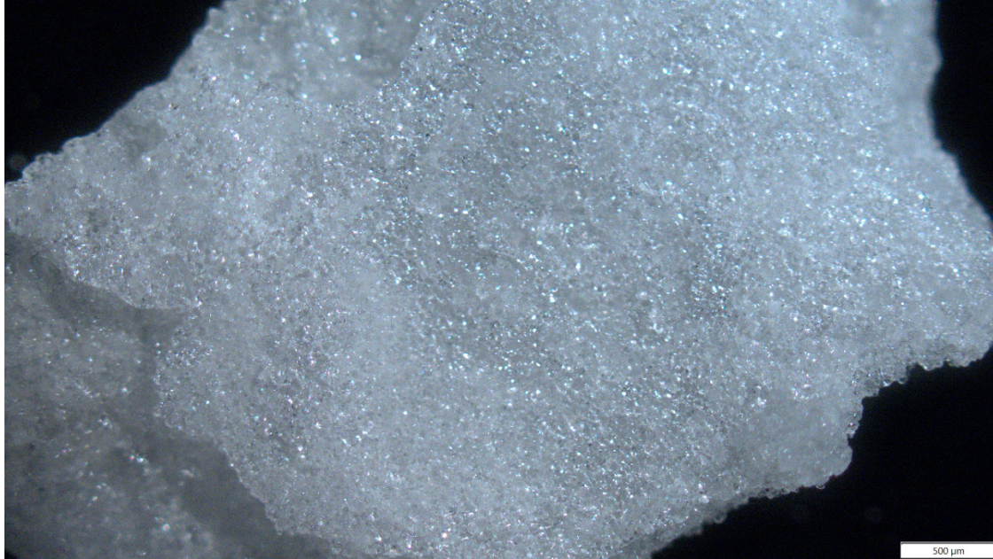
fig. 3: Sample 2, up to 1mm thick compact white crust (DF)
