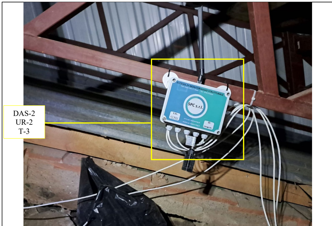
Data Acquisition System - DAS-2, Relative environmental humidity UR-2, Temperature sensor T-3.
