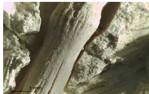
Plant fiber in both plaster layers. 2025
