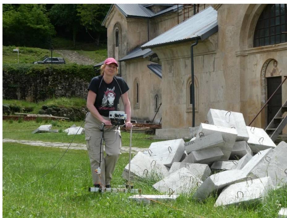
Fig. 4 Gelati. Resistivity prospecting with the Geoscan RM85 resistometer in dipol-dipol configuration. By magnetometer prospecting we covered a survey area covers of ca. 3.200 square m and ca. 4.800 square m by resistivity measurements
