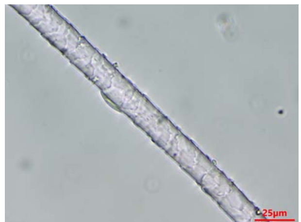
sample 40: wool fibre - microphotographs of the central zone (transmitted light, X polars on the left, // polars on the right).
