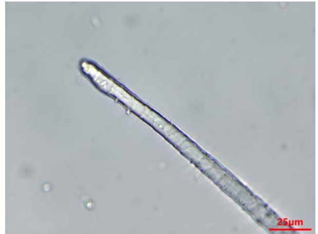
sample 40: wool fibre - microphotographs of root (on the left) and termination (on the right) (transmitted light, // polars).
