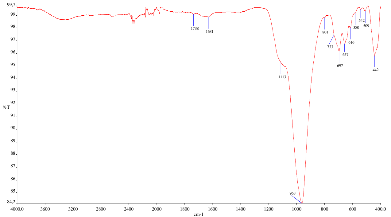
sample 45: FT-IR spectrum of a blue pigment's grain (layer c).
