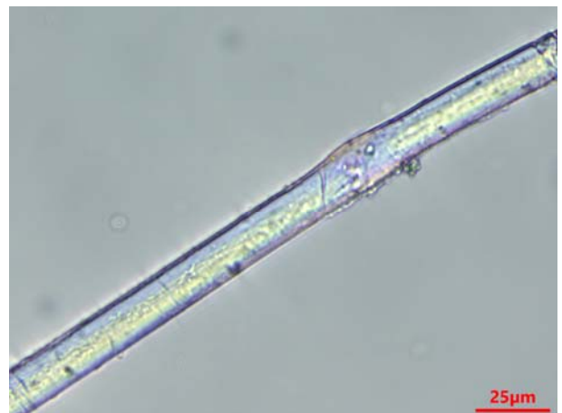
sample 40 – possible hemp fibre: microphotographs (transmitted light, X polars on the left, // polars on the right).
