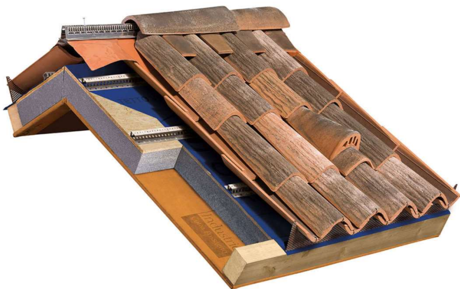
Example for the ventilation system 1. In this case, the covering mantle is made of tiles (from a technical publication).
