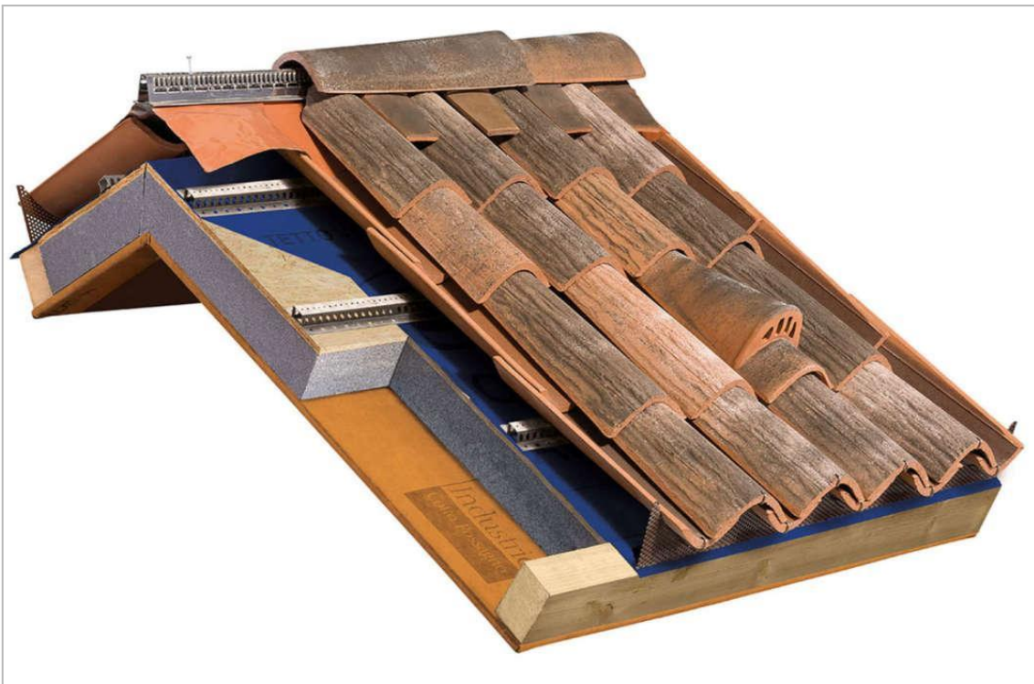
Figure 31 - Example for the ventilation system 1. In this case, the covering mantle is made of tiles (from a technical publication).
