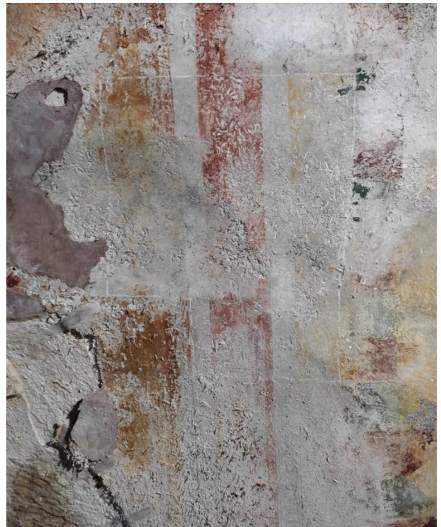
plaster consolidation test with ammonium oxalate
