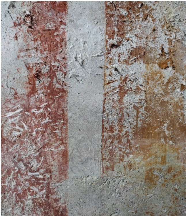
plaster consolidation test with ammonium oxalate
