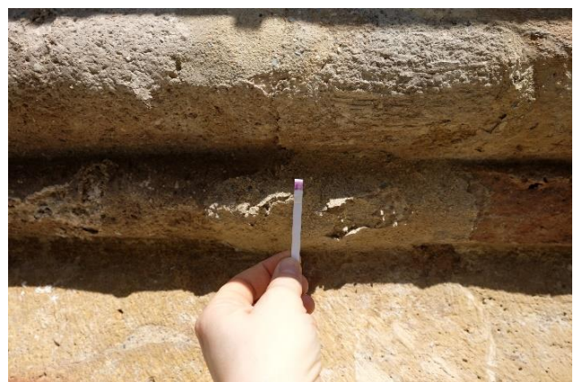
Figure 30: Nitrates check on the cornice (test N29)
