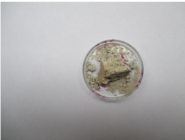
Figure 42: Point GB , sample 30, layer for tiles nailing
