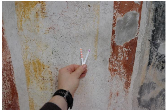
Figure 28: Nitrates and Sulphates check
