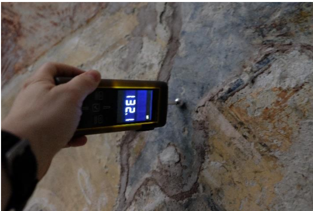
Figure 27: hygrometric measurements by portable instrument
