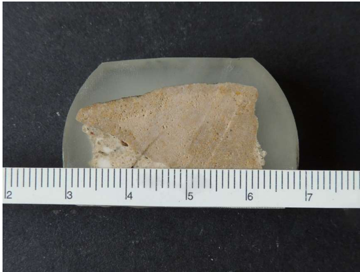
M XVI - Cross section image: the mortar is in the left side
