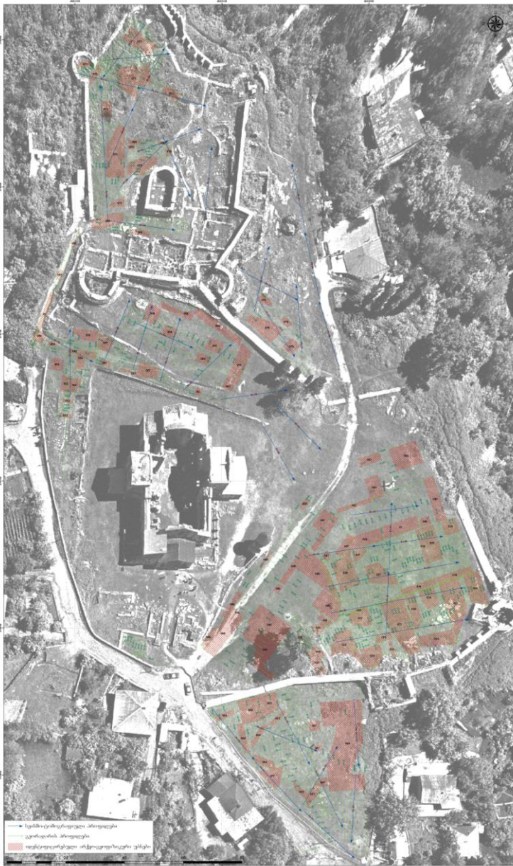
Fig. 3. Survey results: revealed underground disturbances
