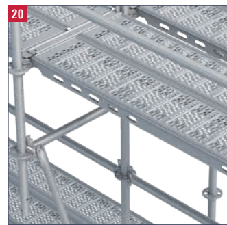
20 Support cantilevers 0.5m below the deck level with bracket braces or Allround diagonal braces. Safeguard scaffolding decks on cantilever structures from being inadvertently lifted out using appropriate lift-off preventer.
